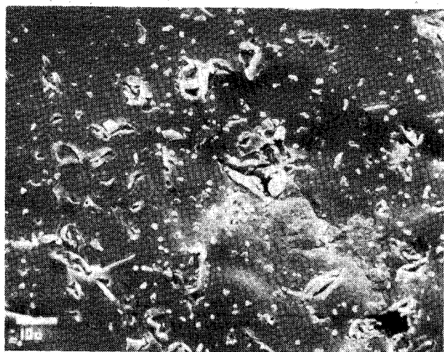
Fig. 5. Micrograph taken at 1000\times showing a particle eroded surface after 50 h of exposure to the oxygen plasma. The appearance is similar to that of Fig. 4. No evidence of undercutting is visible.
